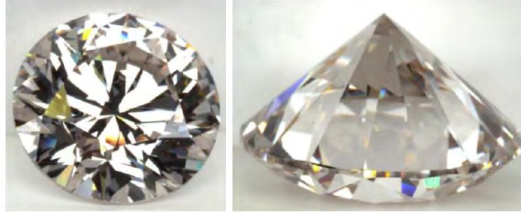
Figure 1: The 3.09 ct CVD lab-grown diamond (brilliant cut) brought to HRD Antwerp for examination.
